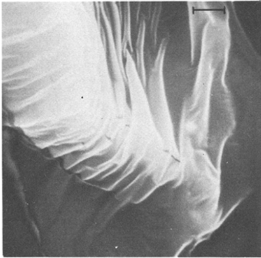
Figure 7 ESC fracture surface, MFI 20 (Scale 2 \mu\text{m} ).
